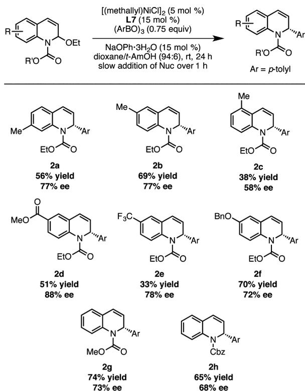
**Figure 3.** Electrophile scope. (a) Reactions run on a 0.5 mmol scale at 0.01 M under an N<sub>2</sub> atmosphere. (b) Isolated yields (average of two runs). (c) Enantiomeric excess determined by chiral HPLC (average of two runs).
