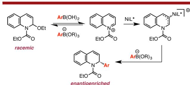
**Figure 1.** Ni–iminium activation mode for asymmetric catalysis.
